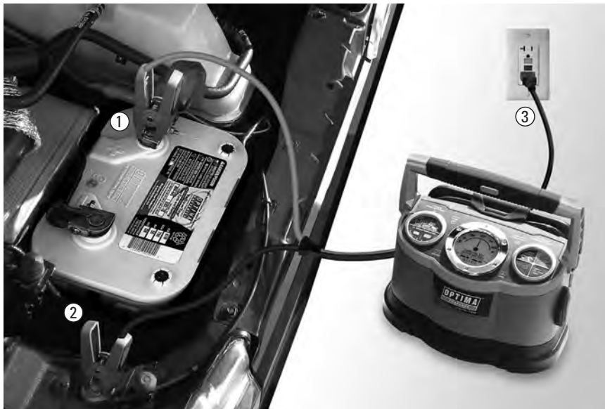
Pictured: Typical DC charging clamp connections for a precharge status (with engine off), charging or just maintaining a fully charged battery with the DC charging clamps in a vehicle.
