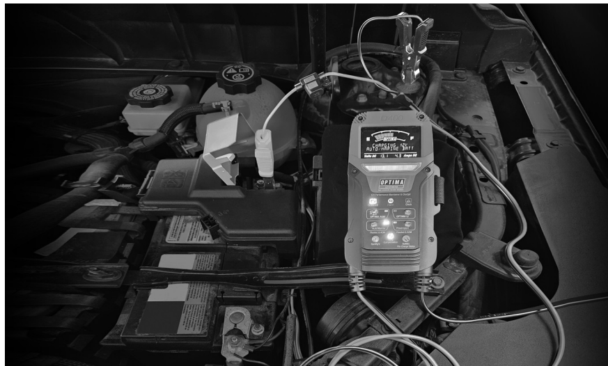
Pictured: Typical DC charging clamp connections for a precharge status (with engine off and charger unplugged from AC power), charging or just maintaining a fully charged battery with the DC charging clamps in a vehicle.
