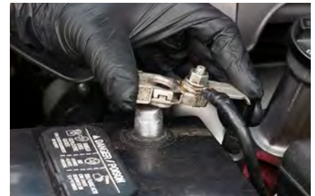
Step 8 - Reinstall the positive cable.
