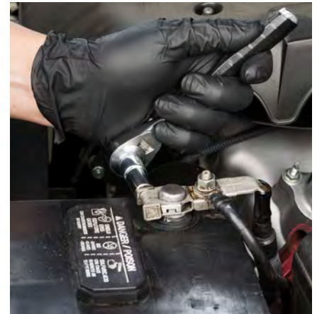
Step 3 - Disconnect the positive cable.
